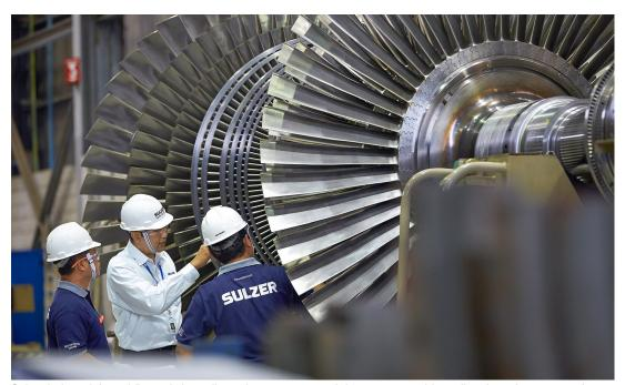
Sulzer Indonesia's mobile workshop allows the teams to repair large steam turbines directly at the customer's site.
